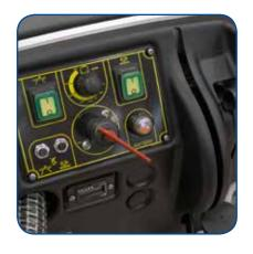
User friendly analogic control panel. Control lever for brush operation and detergent water outflow. ON/OFF and battery cutout key switch, brush and vacuum motor switch, detergent dosing knob (optional), Thermal circuit breaker to protect
